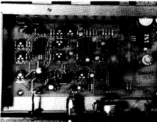
All controls and switches are easily accessible with chassis cover removed. Each is individually labeled for easy identification. Clockwise rotation of pots increases desired function, and vice versa.
