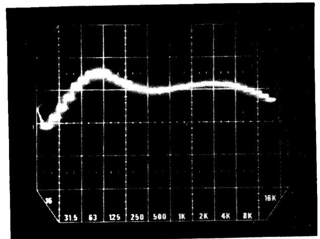
Bass control in full boost position and HF control flat. Helps add bottom end to bass deficient systems. Also, "sweetens" sound. Low limiter setting is employed to keep from limiting bass energy.
