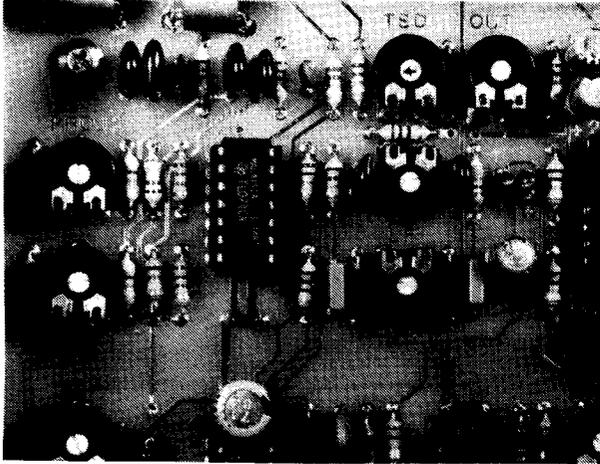
LIMITER THRESHOLD (TSD) and line amplifier control (OUT) are at the top of the PC card. A clockwise rotation increases limiter action and increases output. These two circuits are associated and must be adjusted for compatibility.
