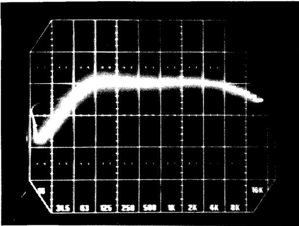
Real time 1/3 octave analysis shows film inputs with bass and HF controls in the flat position. Notice 18 dB per octave high pass filter which cuts frequencies below 50 Hz. This minimizes splice "thumps" and mechanical rumble.
