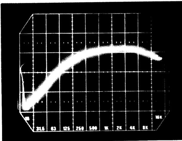
HF control in flat position and bass control at minimum. Useful in highly reverberant acoustic environments such as prisons, gymnasiums, etc. Helps increase intelligibility of dialogue.
