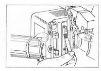
Dirt or dust deposits on the sound heads will degrade the sound playback quality. Clean the sound heads with a cotton swab or soft cloth. In this case, be sure to disconnect the power cord and set the motor switch at "OFF" position.
