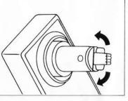
Place your film on the front arm and the take-up reel on the rear arm. Press the reel locks until the reels are snugged against the spindles.
