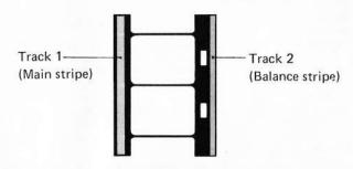
As shown in the left illustration, 8mm sound film is coated with magnetic stripes. Track 1 (Main stripe) is used to carry the sound track when used in conventional sound projectors. Track 2 (Balance stripe), that runs just outside the film perforations, is used to ensure smooth film travel through the projector. The Elmo ST-180EM is a high performance sound projector capable of recording and playback on two sound tracks.
