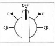
Turn the motor switch to "OFF" position.
