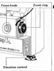
3 Before threading the film, advance the motor switch to " [;" position and project the light on the screen for adjusting the picture position with use of the elevation control.
