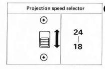
6 Select the proper projection speed, either 24 fps (UP) or 18 fps (DOWN).
