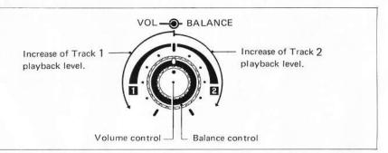
The balance control knob is used to balance the playback levels of Track 1 and Track 2. The balance control is normally set in the middle position. If Track 1 is higher than Track 2, turn the knob clockwise until both tracks are balanced.
