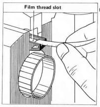
4 Insert the film leader into the thread slot as indicated by the red arrow. The film will automatically thread to the take-up reel through the film guide.
