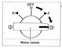
Set the motor switch to " ☐ "position to turn the lamp ON. With this operation, the auto thread lever will release automatically.
