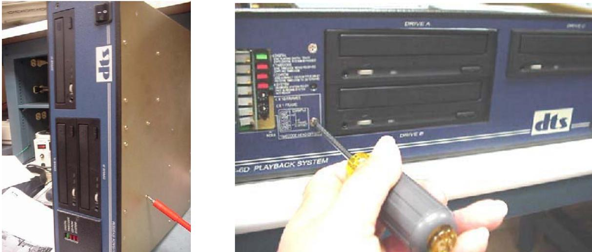
Figure 2. Typical: remove screws on bottom and front panel that secure drive bracket to chassis.
