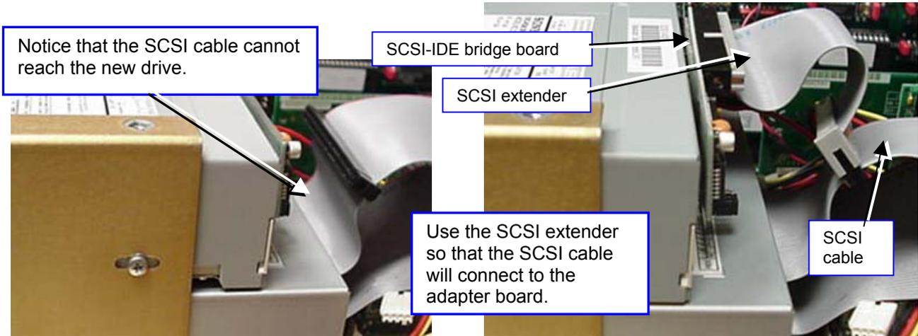
Figure 6. Install the SCSI adapter cable.
