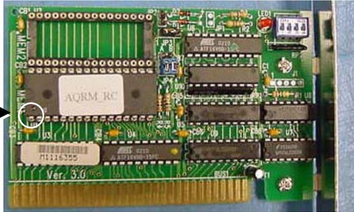
Figure 10. ROM board with AQRM chip
