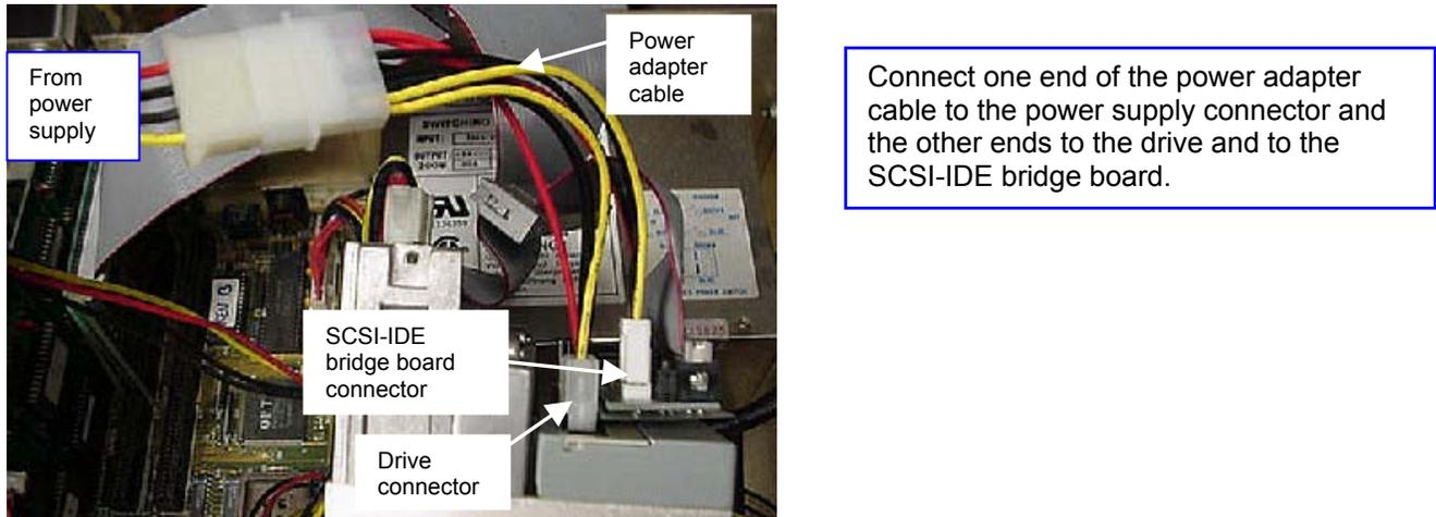
Figure 7. Install power adapter cable.
