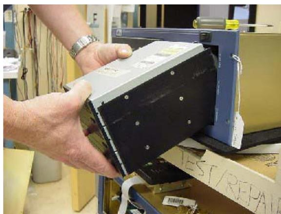
Figure 11. Loosen screw and remove drives
