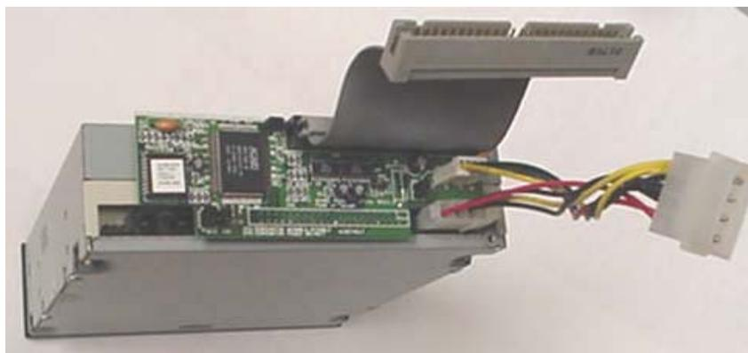
Figure 14. Back of DVD Drive with SCSI-IDE Bridge board, Power Adapter Cable and SCSI extender cable attached.
