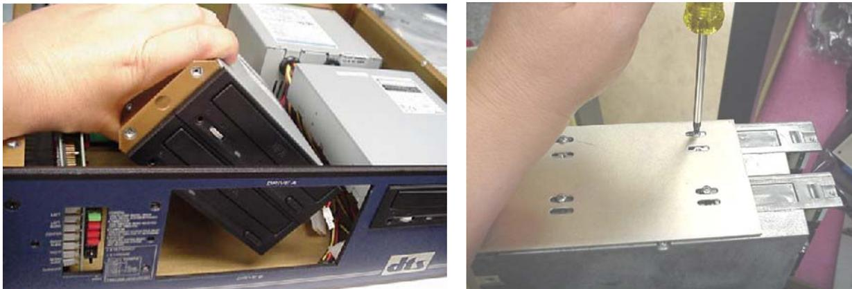
Figure 3. Remove brackets from old drive and install onto new drive.
