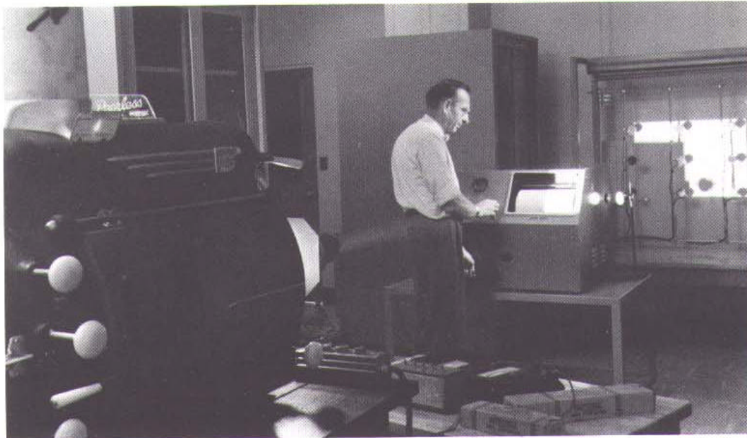
A recording spectroradiometer plots a color output curve in a minute and a half...it previously took half a day.
