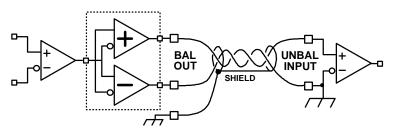
Once again the output signal must be properly terminated at the unbalanced input and the shield must be connected only at one of its ends so as to avoid connecting the two equipment grounds together and creating a ground loop. The cross-coupled circuit ensures that the signal level is properly maintained.
