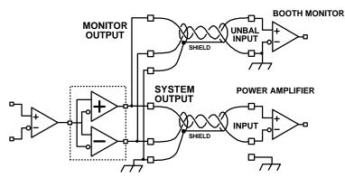
Notice that the unbalanced input of the booth monitor effectively unbalances the output of the DFP-D3000, as it connects the – or "cold" out-of-phase side to the booth monitor's ground. Nevertheless, if the wiring is done as illustrated the power amplifiers will suffer no hum problems. Chassis grounds of all three pieces of equipment will not be connected together by the wiring, and no component of the audio signal flows in shields.
