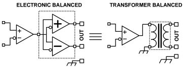
The circuit on the right uses a transformer to connect the output of an internal circuit stage to the outside world while isolating chassis ground from the audio signal. The circuit on the left uses a cross-coupled electronic circuit to achieve the equivalent result: true electronic balancing.
