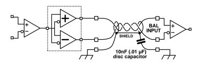
A small disc ceramic capacitor is inserted into the connection between the shield and ground at one end only.
