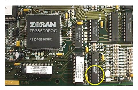
Carefully solder one 10k ohm 5% 0.25W resistor between pins 13 and 10 of IC20 and another 10k ohm 5% 0.25W resistor between pins 15 and 8 as shown on the drawing and photograph below.
