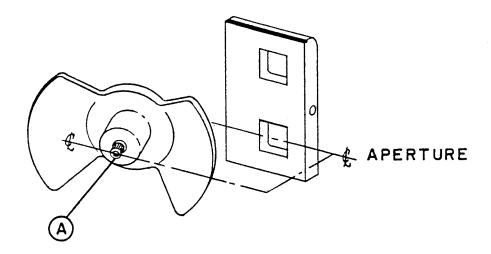
TURN PROJECTOR FORWARD BY MOTOR FLYWHEEL UNTIL SPROCKET TOOTH <sup>#</sup>2 IS AT INDICATOR. LOOSEN SCREW (A) AND TURN SHUTTER SO (L OF BLADE IS ON (L OF APERTURE OPENING.
