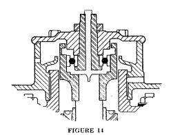
The bearing is in a grease tight housing and the presence of any grease on the outside of the machine indicates clearly that a surplus amount of grease is being forced into the bearings. This surplus grease mixed with carbon dust or dirt will cause serious trouble by grounding the windings of the machine.
