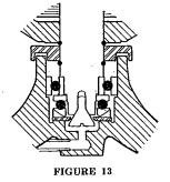
The inner ball race of the annular bearing is held on the shaft by the thrust load. The retainer washer and retainer screw serve to keep the assembly intact when the rotor is removed from the base.
