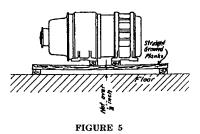
With ball bearing mountings, it is not so essential to have the foundation perfectly level as in the case of oil bearings where the shaft must be substantially horizontal.
