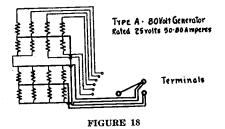
Figure 18 shows the internal connections of one of these rheostats. It will be noted that this rheostat is of the parallel type, the units being wound of nickle-chromium wire and carry 5 amperes each. There is a sufficient number of units connected across the terminals permanently to obtain the minimum current as given in the rating. The adjusting handle gives six 5 ampere steps of increased current.
