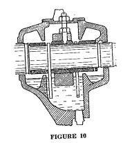
Bronze bushings are used in most of the sizes. They have a free mounting, being supported for only 20 per cent of their length. This allows the bearing to follow any slight deflection that may occur in the shaft. It also permits it to align itself in case of a mis-alignment of end yokes.
