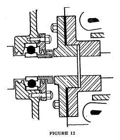
Figure 13 shows the construction of the bottom bearing of the Vertical Transverter. The bearing retainer screw has a left hand thread so that it will not back out in operation.
