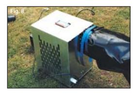
It is vital to cover the fan if the weather is wet outdoors to avoid the fan shorting out. Also do not turn on its side as it may ingest grit or other material from the ground, which will damage it.
