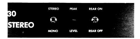
OPERATOR SWITCHES THAT ARE FREQUENTLY USED ARE ON LEFT SIDE OF FRONT PANEL
