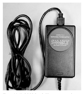
Figure 14. Model PS-2 switching power supply.
