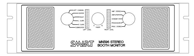
**Listening Modes.** The right knob controls listening mode. When set to AMP STEREO or PROC STEREO, the MN596 sends Left and Center channel signals to the left speaker, and Right and Center channel signals to the right speaker, creating a stereo sound with a "phantom" center channel. The left knob selects the individual channel monitored in the AMPLIFIER and PRO-CESSOR listening modes. STANDBY mode disconnects all monitoring signals, but does not power down the system.
