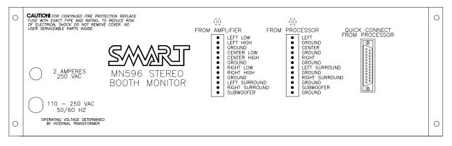
**Connections**. The MN596 has Phoenix connector inputs for amplifier and processor signals, as well as an alternate THX standard DB25 processor connection (see diagram at right). Simply connect appropriate amplifier and processor signals to the indicated Phoenix positions.
