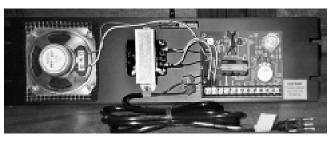
The power transformer connects to the two terminals on the far left. Because the supply delivers 18-20 VAC polarity is not important. Audio signals from the stereo processor are connected to the input terminals for the appropriate channels.
