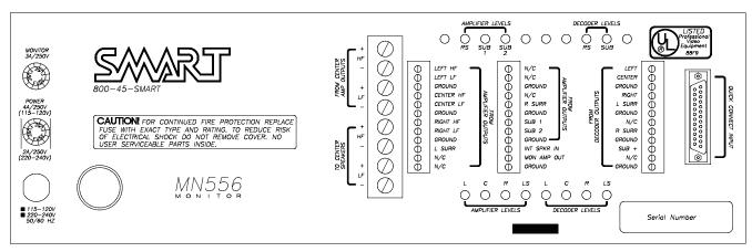
the internal speaker and the monitor amplifier. Connect the external speaker to the "MON AMP OUT" terminal and GROUND. The monitor Fader on the front panel will control the volume to the remote speaker. Both the internal and remote speaker may be used simultaneously by leaving the jumper in place and connecting the remote speaker to the "MON AMP OUT" terminal and "GROUND", as long as the remote speaker has an impedance of 8 ohms or more.
