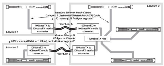
\*Although any one fiber segment can be up to 2000 meters long, and any single UTP segment can be up to 100 meters long, it may be necessary to impose shorter limits, in consideration of cumulative delays caused by devices and cabling. See text for more information.
