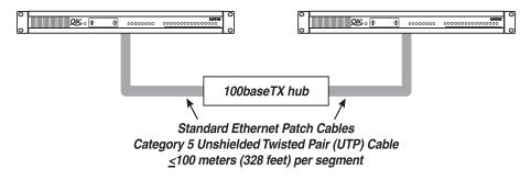
This network is similar to the previous one, but with a hub in between, breaking up the network into two segments which can each be up to 100 meters long. Yes, there is the added expense of a hub, and you are adding the slight possibility of a hub failure, but the net media can be simple off-the-shelf patch cables, and you can easily expand the net-
