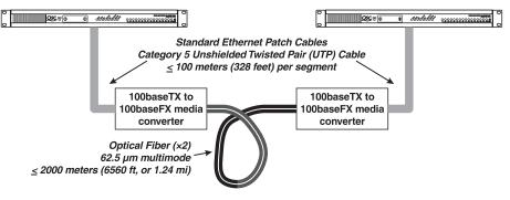
Likewise, the other network topologies described here earlier can be upgraded with optical fiber. This can be done with media conversion on individual network segments, as shown here, or by using fiber to interconnect hubs (illustrated on the following page), or combinations thereof.
