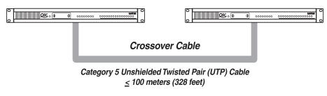
The simplest and most direct RAVE network comprises two RAVE units connected by a single crossover cable. This network has only one segment, so the 100-meter limit applies to the segment and thus to the entire network. There are no hardware costs other than the RAVE units themselves and the cable for
