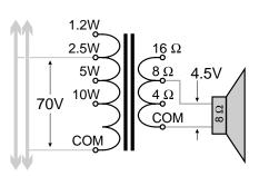
Example of a loadspeaker connected to a distributed line through a transformer
