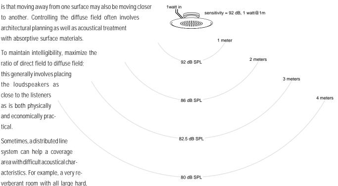
reflective surfaces—wood floors and ceiling, concrete and plaster walls, etc., the type of room that tends to make speech unintelligible—might benefit from using many low-powered loudspeakers placed throughout the room and close to the listeners, instead of using a couple high-powered, centrally-located loudspeakers.
