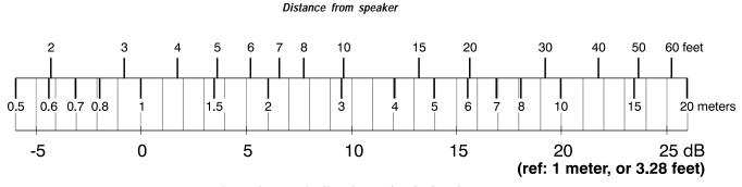
Power increase in dB; referenced to loudspeaker sensitivity rating (1 watt @ 1 meter)
