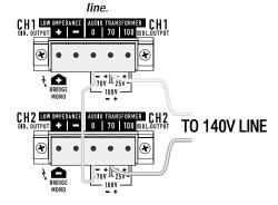
Output connections for CX, parallel or stereo mode.
