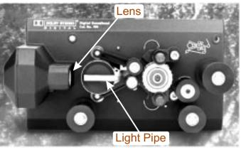
Caution: Never remove the reader assemblies without the proper alignment equipment.
