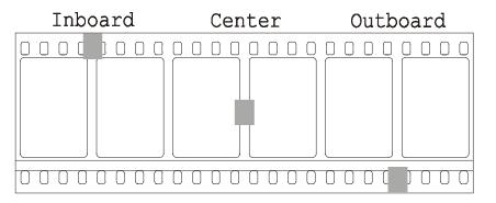
Little or no maintenance is required other than Keeping the optical assemblies clean. The Film Presence and Film Motion detectors operated by shining infra-red light onto the film and then detecting the light when it is reflected back. If the L.E.D.s from which the light comes, or the phototransistors which receive it, get too dirty, the detectors can't work. In a normal cleanly maintained projector it is usually sufficient to merely wipe the optical area with a clean dry cloth.
