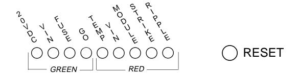
WHEN ALL FOUR of the green indicator lights are glowing, the power supply is operating trouble-free. One or more red lights, when glowing, indicates that a problem exists, and disables operation of the power supply. The red light(s) latches and remains glowing until the RESET button is depressed after the problem has been corrected.
