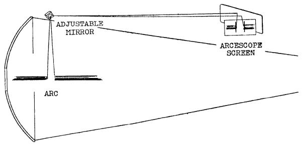
EXACT ARC FOCUS and proper arc gap length are assured after the arcescope has once been set, by simply maintaining the images of the burning carbon tips at these arcescope lines.
