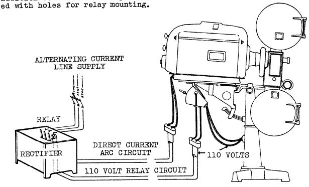
A 30 AMPERE FUSED KNIFE SWITCH should be connected to the alternating supply circuit just ahead of each rectifier so that all of the equipment will be dead when the switches are open.
