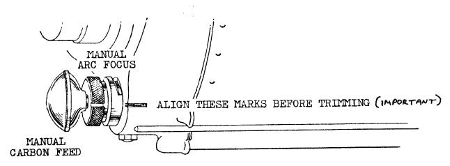
PRELIMINARY ADJUSTMENT OF LIGHT to the screen may be made while the projector is running but without film. However, the final reflector focusing is best done while projecting a picture.
