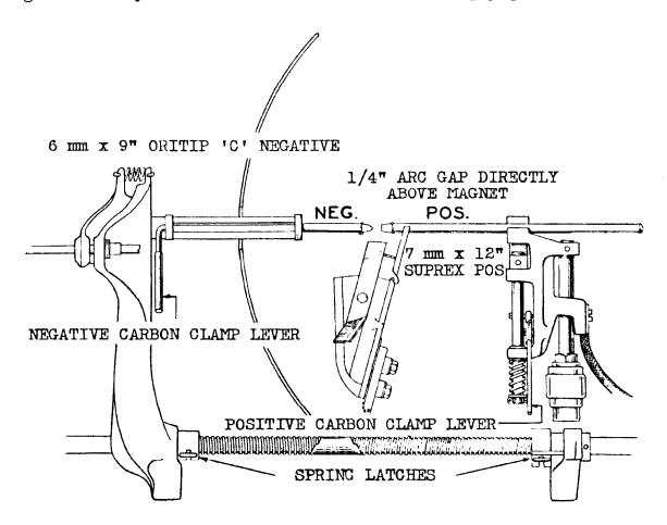
TO TRIM THE LAMP clamp the 7 m.m. carbon in the positive holder and the 6 m.m. in the negative holder. There should be a 1/4" gap between the positive and negative carbon tips and this gap should be directly above the tips of the supplemental magnets. This location of the carbons will assure approximate focus when the arc is first struck.
