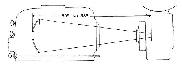
THE OPTICAL ALIGNMENT of the lamphouse with the film aperture should be checked by inserting the aligning rod into the fully separated carbon holders. A rod is supplied with the lamps.
