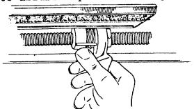
SEPARATE THE CARRIAGES that carry the carbons, to the full limit of their travel, by depressing their spring latches with the thumbs of each hand. This downward pressure will disengage the carriages from the carbon feed screw so that the carriages will slide freely along the carbon feed screw and guide rods.
