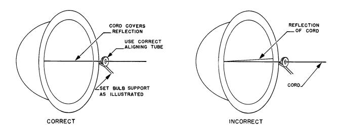
ALIGN THE LAMPHOUSE in relation to the projector so the cord passes through the center of the hole in the test aperture, and the correct cord image is seen on the reflector. Set the anode support yoke as illustrated and tighten the set screw in the air duct. DO NOT reposition the reflector, as it is factory prealigned for maximum optical efficiency.
