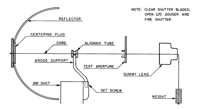
POSITION THE LAMPHOUSE on the table so the center of the reflector measures as near 34.5 inches from the projector aperture as the projector design will permit.
