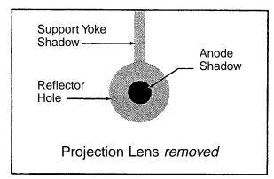
MOVE THIS CONTROL SECTION around the two thumb screws until the black spot is as round as possible to project. It may be necessary to again adjust the focus control to define a sharp spot. After the black spot is as even as possible to project, tighten the two thumb screws to lock the adjustment section. This adjustment has now centered the projected image of the electrode shadow and the hole in the reflector on the aperture and screen.
