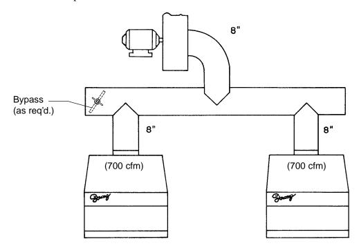
CHECK EACH LAMPHOUSE for correct exhaust air flow. Insufficient exhaust draft can severely shorten bulb life, and **no credit** will be allowed bulbs damaged in this manner. Inadequate exhaust may also cause possible injury to personnel by overheating the lamphouse enclosure.
