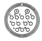
Modification for use with Spotlight or other non-console lamphouse: Remove the jumper from between Pin E & F; remove black lead from Pin C and relocate to Pin F. This will supply 110 V.AC to the main board for the **GO** light.
