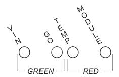
WHEN BOTH of the green indicator lights are glowing, the power supply is operating normally and trouble-free. A red light, when glowing, indicates that a problem exists, and disables operation of the power supply.
