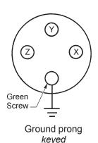
A four-prong, female plug is furnished to mate to the AC receptacle mounted to the power supply. Connect 208/230 V.AC three phase input to terminals X, Y, and Z. Connect single phase input to terminals X and Z *only*. Single or three phase neutral is not required for installation of this unit. Attach an adequate earth ground to the green ground terminal.
