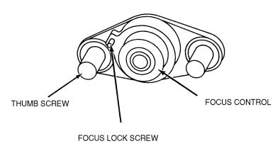
THE THUMB SCREWS on either side of the focusing control lock the horizontal and vertical adjustment mechanism in position.
