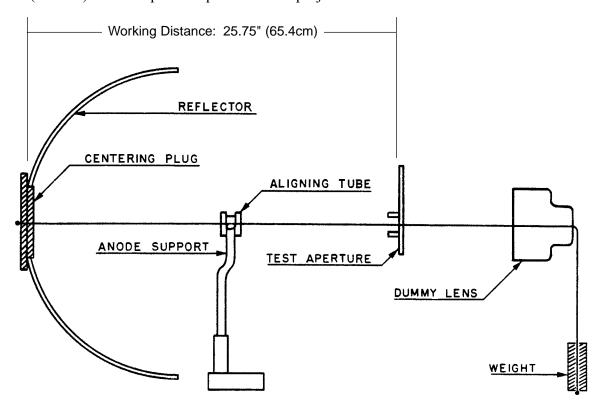
WITH A XENON PROJECTION LAMP it is **imperative** that the lamphouse optical system is aligned exactly with the projector optical center in both the vertical and horizontal planes.
