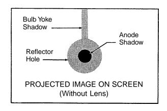
MOVE THIS CONTROL SECTION around the two thumb screws until the black spot is as round as possible to project. It may be necessary to again adjust the focus control to project a sharp spot. After the black spot is as even around the outside as possible to project, tighten the two thumb screws to lock the adjustment section. This adjustment has now centered the projected image of the electrode shadow and the hole in the reflector on the aperture and screen.
