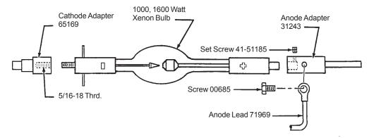
ASSEMBLE THE ADAPTERS to the 1000 or 1600 watt bulb prior to removing the plastic protective covering. DO NOT apply mechanical stress to the quartz envelope. Firmly tighten all fasteners before installing bulb and adapters.
