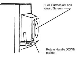
ALL CONSOLE front castings are drilled and tapped to accommodate field installation of the Beam Expander Kit. The nose cone can be trimmed with tin snips to fit as required without disturbing the 33-1/8 inch working distance of the lamphouse reflector to the projector aperture.
