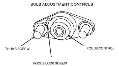
THE CENTER SECTION of the control is a threaded member that focuses the bulb in relation to the reflector. Turning this adjustment moves the bulb in only one plane, into or away from the reflector. Clockwise rotation moves the bulb away from the reflector. The small knurled screw to the left of this section can be tightened to lock the focusing mechanism, after the following procedures have been completed.
