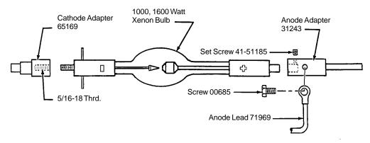
ASSEMBLE THE ADAPTERS to the 1000 or 1600 watt bulb prior to removing the plastic protective covering. DO NOT apply mechanical stress to the quartz envelope. Firmly tighten all fasteners before installing bulb and adapters.
