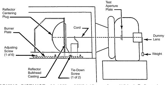
WORKING DISTANCE: 33.125" ± .25"/84.15cm ± 6mm (15 inch Reflector) 27.75" ± .25"/70.5cm ± 6mm (12.8 inch Reflector) Distance between "Centering Plug" & "Test Aperture Plate" = *Working Distance*
