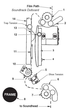
Unlatch and open the turret. Rotate the framing knob (Item 8) to its center position (FRAME reading level, as shown). Using the soundhead flywheel, turn the mechanism by hand to rotate the intermittent sprocket (Item 9) to its "rest" position. In the "rest" position, the index mark (Item 10) will align with one of the painted white index lines on the intermittent shaft collar after the sprocket has completed a four-perforation step.
