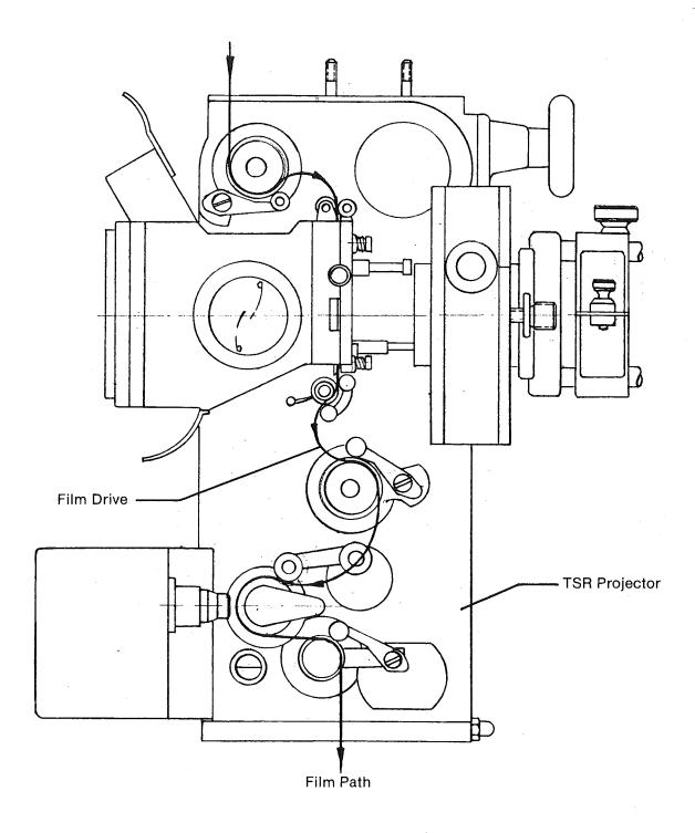
Fig. 5-3: Threading Diagram
