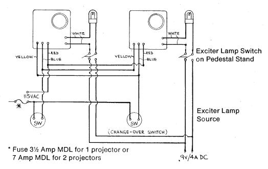
4-2: Connection Diagram for Changeover Switch
