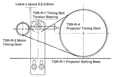
Fig. 6-4: Timing Belt Tension Bearing Setting Point
