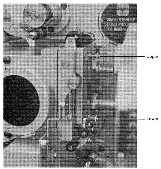
Fig. 5-6: Gate Pad Adjustment Collars
