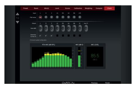
The Check step allows you to verify and adjust SPL if necessary. The Optimizer will set the screen channels at 85dB and surrounds at 82dB (-3dB on the settings). Subwoofer(s) will be between 87-90 dB. It is also possible to monitor the output channels on Aux1/Aux2 and setup the associated volume.
