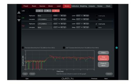
Here we see the Power and Direct response. With perfect timing, you will see the least amount of dip in the frequency response. There is a possibility to fine tune this Time using Power and Direct graphs to guide you. This is covered in an advanced document. Link here\*.
