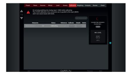
This shows the calibration process. It will measure each channel. Best measurements are taken between 80-90dB (85 being ideal). Sub will be louder of course. So, the mic level with be less stable for sub.
