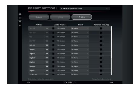
The "Profiles" tab is showing the whole profile list available. Each one can modify the volume and load aspecific preset when we activate it. It is possible to define a profile to load up at boot by
