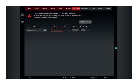
When the measurement cycle is finished, you should see a green "Calibrated" under status.
