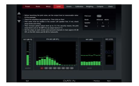
Here is the HF and LF together relatively balanced and at 65dB
