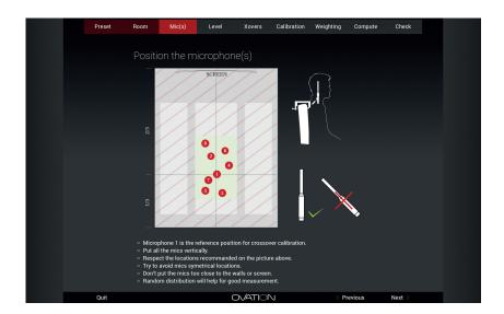
This page is an explanation of microphone placement and orientation.
