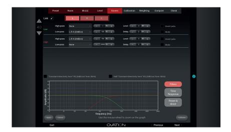
You can link your parameters between speakers with the same amount of channels. In this example, L, R and C will have the same value settings.
