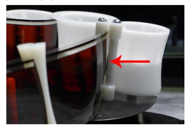
In addition to the concern of scratching on the right stripper post, as the film curls just a little bit more, the film will then scratch on the payout arm's "wishbones" as the edges of the film press up against one wishbone forcing the image area to press into the other wishbone. The below procedure will prevent the scratching.
