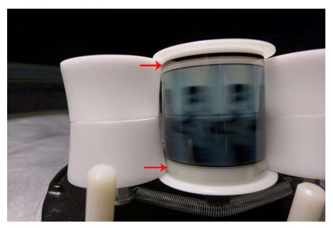
This is the brain in action after performing ALL of the above modifications. Please note you MUST thread to the RIGHT side of the existing (left) stripper roller, just as you would if the (right) stripper roller that you removed was still there, otherwise erratic payout and overall wackiness will ensue.
