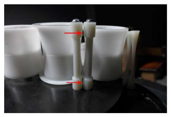
Next inspect the alignment of the two stripper rollers in relation to where the image area of the film is riding. Below is a typical picture showing misalignment that can cause scratching at the point of the arrow.
