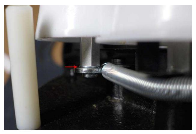
Similarly, if the film is riding "too low", the washer(s) can be added below the stripper posts to correct for the alignment problem.
