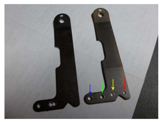
Now re-mount the two wishbones in the new "medium" position using the original BLUE hole and the newly created YELLOW hole. (Note the photo above with the arrows was taken looking at the UNDERSIDE of the arm.)
