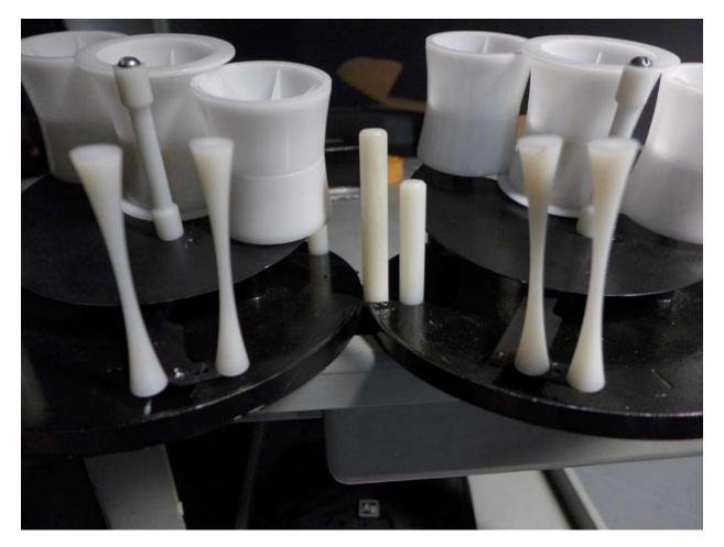
Finally, before using your modified brain, ensure the two flange-less rollers are making even contact with the flanged center roller as seen with the two red arrows for the left roller. If for example only the bottom edge of the flange-less rollers are making contact, your film COULD walk right up and out of the brain during operation. If you find this is an issue with your brain, the only solution is to gently bend the shaft slightly so it lands squarely on the center roller.
