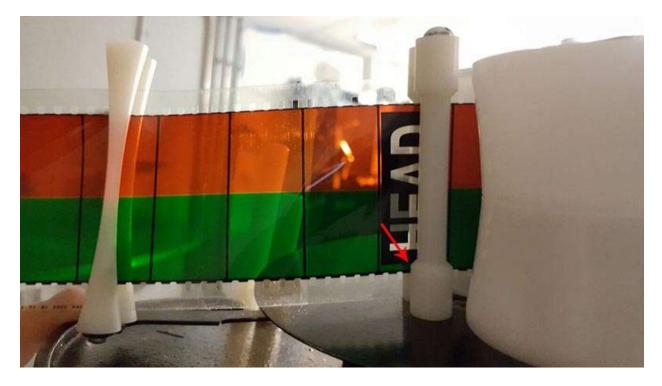
To prevent this misalignment from scratching, washers can be used. If the film is riding "too high" as in the picture above, a washer (or two or three) can be placed underneath the roller's shaft like is seen in this picture.
