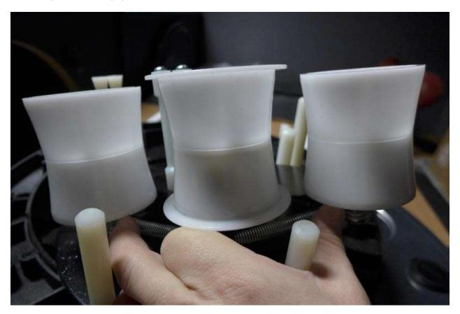
This is how the alignment should look once correct. Note the stripper posts are ONLY coming into contact with the sprockets outward.
