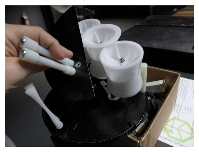
Now remove the stripper base plate entirely. Don't lose the bolt.
