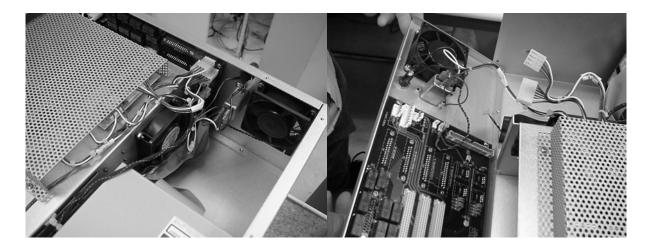
⑤ If the DTS-6AD is first generation (display held by top latch), you will have to drill holes in the rear sides of the sub chassis for the new back panel to fit. The holes are needed for the study to poke through.
