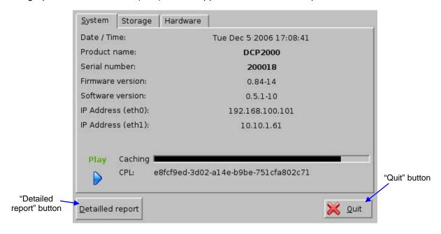
Figure 1: Diagnostic Tool Graphical User Interface (GUI)
