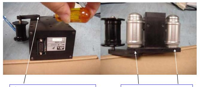
One set-screw to secure auxiliary roller
