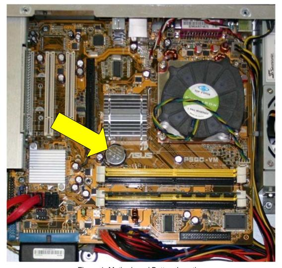
Figure 1. Motherboard Battery Location
