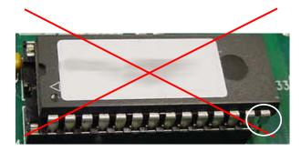
Chip is not aligned correctly with socket. Pin is outside socket.
