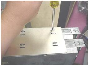
Figure 3. Remove brackets from old drive and install onto new drive.
