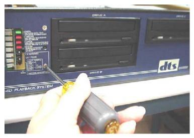
Figure 2. Typical: remove screws on bottom and front panel that secure drive bracket to chassis.
