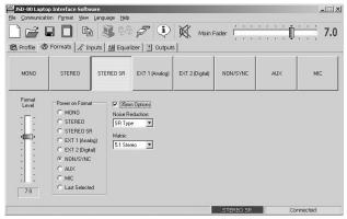
The MONO, STEREO A, STEREO SR buttons can be configured with the following noise reduction options: "None," A Type, SR Type. The same buttons can also be configured with the following matrix decoding options: "5.1 Stereo," "2.0 Stereo," or "Mono." The 5.1 stereo option is the default setting. The 2.0 stereo option is for either Left/Right stereo or Center/Surround systems.
