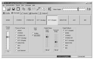
The EXT 2 button can be configured either for "AES-EBU" (Digital) or "Analog" inputs.
