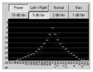
8. Using the built-in Slit EQ Analyzer, run a pink noise test film (Cat 69P or equivalent). Adjust the focus of the soundhead optics for the best high frequency response on the analyzer (see below). At the same time, adjust the azimuth for the thinnest display on the oscilloscope. The focus and azimuth adjustments interact, so it will be necessary to keep adjusting both until the best combination is achieved.
