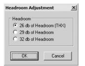
Select one of the three settings. Generally, 26 dB of headroom is sufficient provided there is not more than 6 dB total boost between bass and low frequency 1/3 octave filters or between treble and high frequency 1/3 octave filters. For instance, if the bass slider is set at +3 dB and any of the 1/3 octave eq bands from 40-125 Hz are boosted more than 3 dB, the headroom will be compromised.
