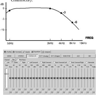
3. Adjust the equalizer sliders until the response shown is obtained. Please note that once a slider is selected with a mouse click, the cursor pad up/down keys will adjust the slider. The left/right keys will select the adjacent 1/3 octave slider. Use the bass and treble sliders to achieve the overall shape of the auditorium response. After making the
