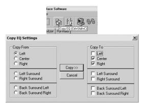
4. Repeat the tuning procedure for the center, right and additional channels. The JSD-80 includes a copy feature that minimizes the time required for this.
