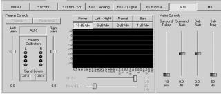
4. Select the Formats tab and select Mic. Click the appropriate radio button to direct the Mic to center or surround channels.
