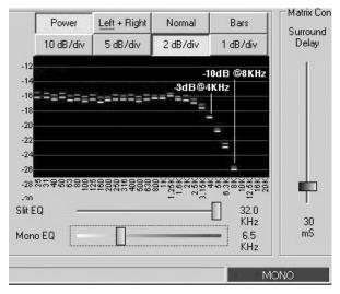
1. Click on the INPUT tab and select MONO format. Thread a pink noise loop on the projector. Using the SLIT EQ Analyzer, adjust the MONO EQ until the above curve is achieved.
