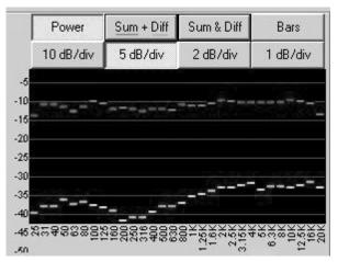
The top graph is controlled primarily by the focus of the reader. The bottom graph is controlled primarily by the azimuth.
