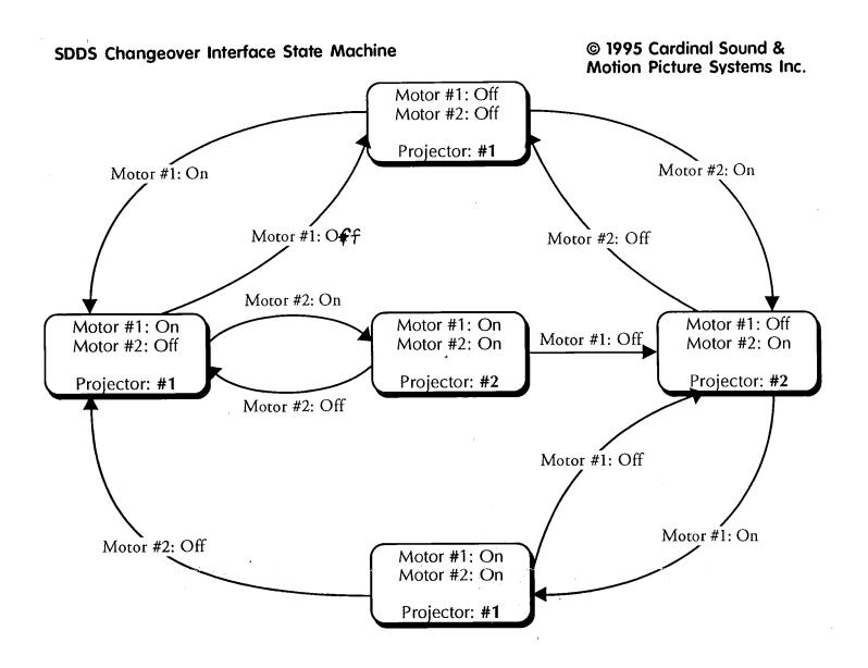
"Projector: #1" means relay "K1" is not energized so the SDDS unit will go to Projector #1.
