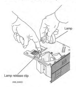
Insert the new lamp into the socket. Push down to tightly seat the replacement lamp. Do not use the clip to seat the lamp.
