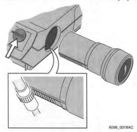
To remove the lens, push the horizontal knob toward the top of the projector as you withdraw the lens.
