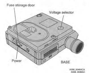
A 220, 230, or 240 main requires a 2.5 A H/250 V fuse. The 100, 115 or 130 V main requires a 5 A slow blow/250 V fuse. To fit or check the fuse, pull out the fuse holder located beneath the power main.
