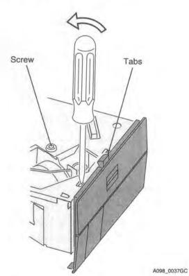
Lift off the top of the lamp module.
