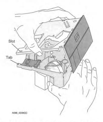
Insert the remainder of the tabs into slots until all seven tabs on the top and two on the bottom are secured.
