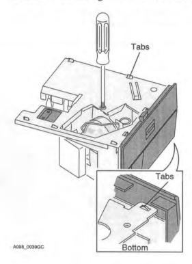
When your maintenance is complete, push the lamp module back into the projector.
