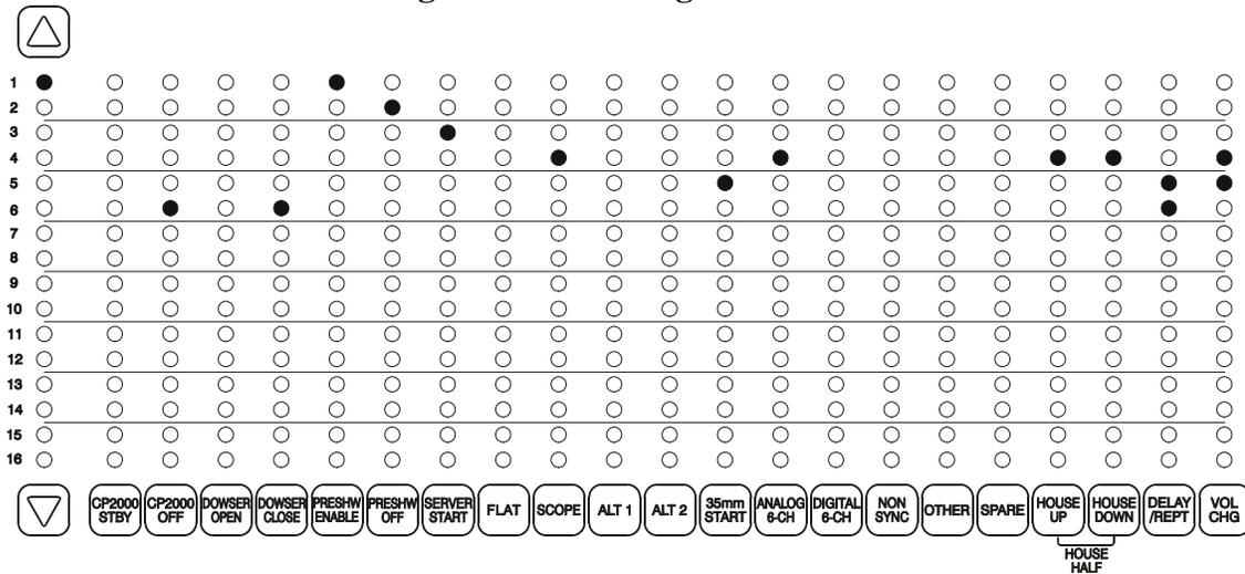
On the left of the panel is a single column of LEDs numbered from 1 to 16, with an arrow key at the top and bottom. These LEDs indicate the step which is currently selected. The step selected in the diagram is number 1.
