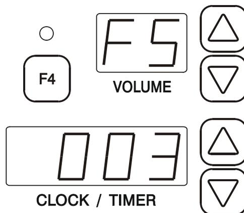
Each setup function is identified in the volume display by a two-character code. Pressing the volume arrow keys will step through the various functions which are available.
