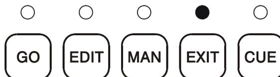
The key labelled CUE can be used to generate a cue manually when a session is running. CUE is also used sometimes as an enter key, for example when setting the time of day clock.
