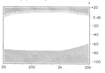
The limits of unassisted analog recording, using a standard professional recorder and tape at 15 ips, are sketched in Figure 1. The limit at high signal levels, actually a gradual overload, is at the top of the clear area. The noise level is the bottom of the clear area. Both the overload level and the noise vary with frequency. The central, open part of the sketch can be thought of as a window through which the signal must fit if it is to be recorded.
