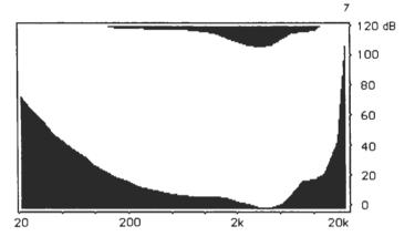
One way to define ideal sound reproduction is to show the limits of the human hearing system as a window, as we did for analog tape recording in Figure 1. Such an auditory window is sketched in Figure 7. The top of the graph corresponds to 120 dB, a continuous sound pressure level that is unbearably loud; at 5 kHz, sound changes to pain at about 110 dB. It is safest, of course, to leave a margin between such a level and the highest continuous sound level one aims at reproducing.
