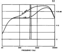
If the signal increases in any part of the spectrum, some adjustment of gain must be made to ensure that overload will not take place. This is done in a very gradual way by Dolby SR, so gradual that there is no danger of producing audible modulation of the signal or any other audible effect.
