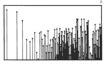
A music program constantly changes in level and frequency content. A moment in such a program might have the spectrum shown in Figure 2. The signal level varies with frequency. The gain setting that would give the best recording at middle frequencies would cause the high frequencies to overload. One objective of Dolby spectral recording is to achieve as nearly optimum a level as is possible at all audio frequencies.
