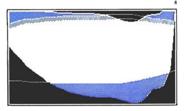
We can learn more about tape recording by superimposing the analog tape window on top of the auditory window. Sliding the analog window up or down corresponds to playing a tape at higher or lower level. In Figure 8 we have set the playback gain so that the maximum level signal that can be put on the tape lines up with a continuous sound pressure level of 110 dB. We will stay with that setting as we look at various recording system windows.
