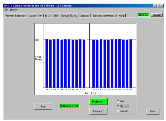
• Now, adjust **PROJECTOR 1** LEFT HF trimpot to achieve flat response from 1 kHz to 12.5 kHz for the left cell.
