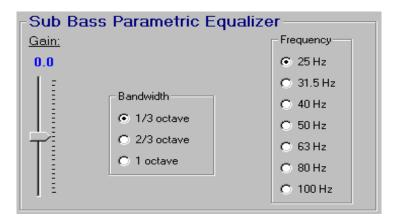
**NOTE:** The DTS-ECP responses slowly to EQ gain adjustments, so give it a few seconds to finish the measurement.
