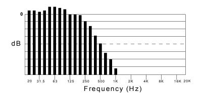
• The **BANDWIDTH** is determined by looking at the width of the area in need of adjustment. In the above example, notice the area needing adjustment is between 63dB and 125Hz. This is one octave, so in this case, select 1 OCTAVE. If the range needing adjustment was smaller, then choose 2/3 OCTAVE. If only a spike appeared, then try 1/3 OCTAVE.
