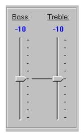
• Do a coarse adjustment to the LEFT TREBLE. Use the cursor to move the adjustment bar up or down, as needed. Adjust TREBLE to achieve a flat response to 2 kHz with the level dropping off 3 dB per octave above 2 kHz on RTA, see below "Standard X-Curve". Click cursor on UPLOAD SETTINGS to send calibration information from the laptop to the DTS-ECP. NOTE: The DTS-ECP responses slowly to EQ gain adjustments, so give it a few seconds to finish the measurement.
