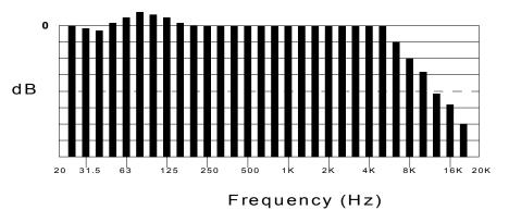
• When the filter has been correctly set, the pattern on the RTA should look the graph below:
