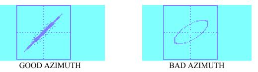
• If the display is not correct, the alignment of the optical head should be checked and mechanically adjusted. Once any changes are made to the solar cell alignment, the optical gain and slit loss adjustment must be repeated.
