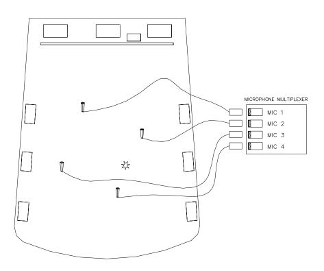
☆ MAKE ALL SPL READINGS AT THIS LOCATION. IF USING A SINGLE CALIBRATED MICROPHONE FOR ADJUSTING EQ, LOCATE THE MIC AT THIS LOCATION.
