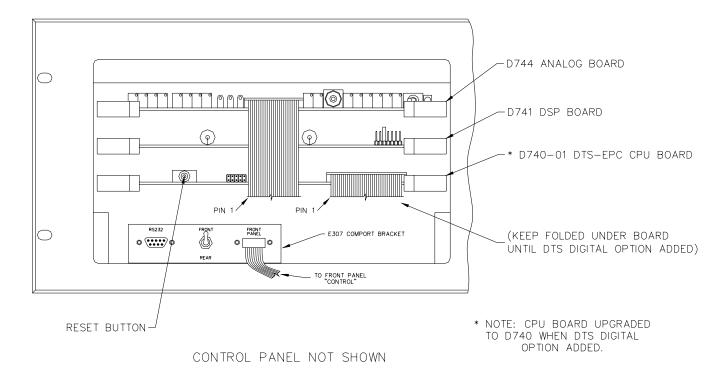
There are two **RS232** ports on the DTS-ECP. One is located on the rear panel and the other on the COMPORT panel, shown above. Both perform the same function of interfacing the DTS-ECP to a PC. Using a null modem cable, connect the serial port of your PC to either the front or back RS232 connector. Use one or the other, do not use both at the same time. After the DTS-ECP is fully booted, you may now start the DTS Upload/Download program **or** the DTS CP Setup Software program on your PC.
