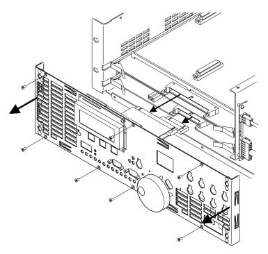
7. Remove the Cat. No. 794 upgrade kit board from its anti-static bag and plug it into the **left-hand** side of the main board by aligning the two connectors shown in the figure. Press down on each side making sure the connectors are fully seated. The board can be oriented only one way for the connectors to match.
