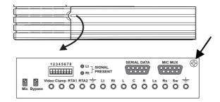
3. Remove the front-panel mounting screw located in the upper right-hand corner of the setup control panel, and carefully pull the front panel toward you to remove it.
