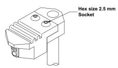
4. Carefully turn over the assembly and loosen the two screw terminals, and remove the wires. Note the wire colors and terminal locations.
