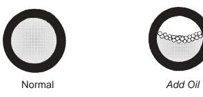
Rotate the motor flywheel by hand to turn the projector mechanism. It should turn freely and smoothly. Start the projector motor and run for at least one minute. Check for an oil splash against the gear compartment cover glass.
