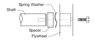
The sound reader flywheel is dismounted for shipping to avoid damage to the impedance drum shaft. Assemble the flywheel to the end of the impedance drum shaft using the wave spring washer and spacer in the sequence shown (spring washer against the flywheel, spacer next to bearing seal). Secure the flywheel to the shaft with the 1/4 inch hex head screw. Note *LEFT-HAND THREAD;* turn *counterclockwise* to tighten.
