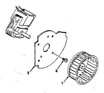
Figure 3-18. MOTOR AND PLATE ASSEMBLY .
