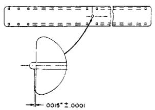
This gage is a piece of stainless steel with perforations simulating double-perforated 16mm motion picture film. This gage is used to adjust the stroke of the projector. The projector functions as an optical comparator when this tool is used.
