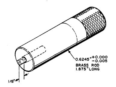
Used to locate the lateral and rotational position of the sound drum.
