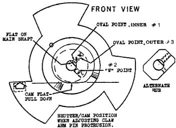
Figure 3-57. SHUTTER AND CAM POSITION
