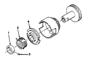
Figure 3-22. CLUTCH ASSEMBLY
