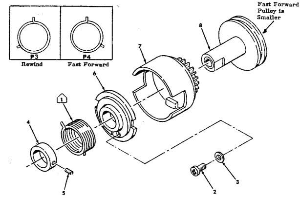
Figure 3-87. REWIND and FAST FORWARD CLUTCH REASSEMBLY
