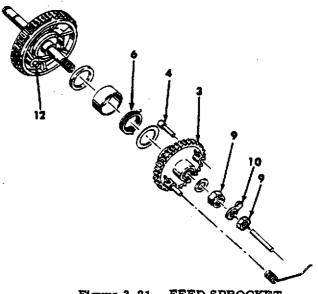
Figure 3-21. FEED SPROCKET CLUTCH COMPLETE
