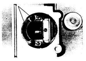
Figure 3-63. ADJUSTING PRESSURE SHOE.
