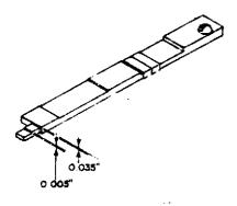
Used to set claw pin protrusion electrically.
