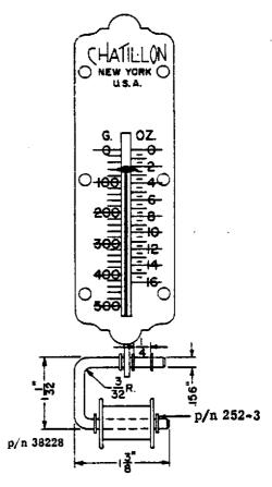
Used to measure forward take-up tension, belt tension and fast forward take-up tension. The scale reading is twice the actual film tension.
