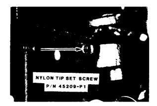
Figure 3-72. REMOVING SOUND OPTICS SETSCREW
