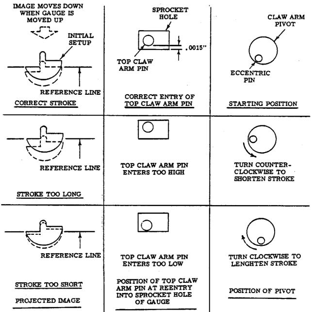
Figure 3-75. CLAW PULL DOWN STROKE ADJUSTMENTS
