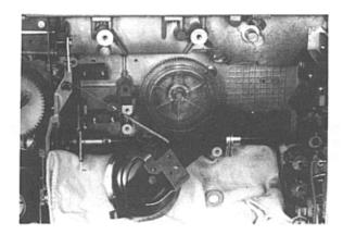
Figure 3-37. CHECK and CLEAN GEARS and BEARING
