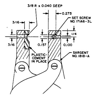
Figure 3-3. ROLLPIN-INSERT AND EXTRACTING TOOL, No. T-38000-N
