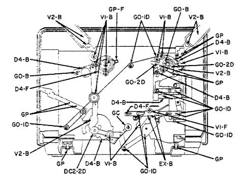
Figure 3-91, Overhaul Maintenance Lubrication Point Diagram
