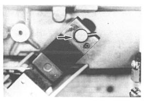
Figure 3-34. ROLL PIN IN POSITION
