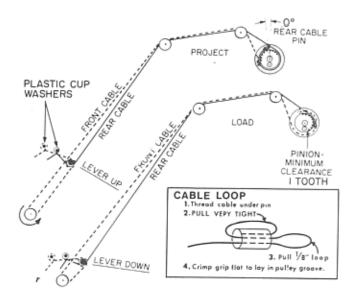
Figure 3-23. CONTROL CABLES
