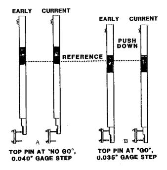
Figure 3-56, CLAW PIN STEP GAUGE READING
