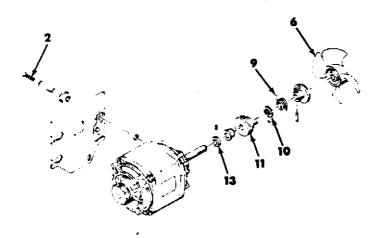
Figure 3-19. DRIVE UNIT ASSEMBLY
