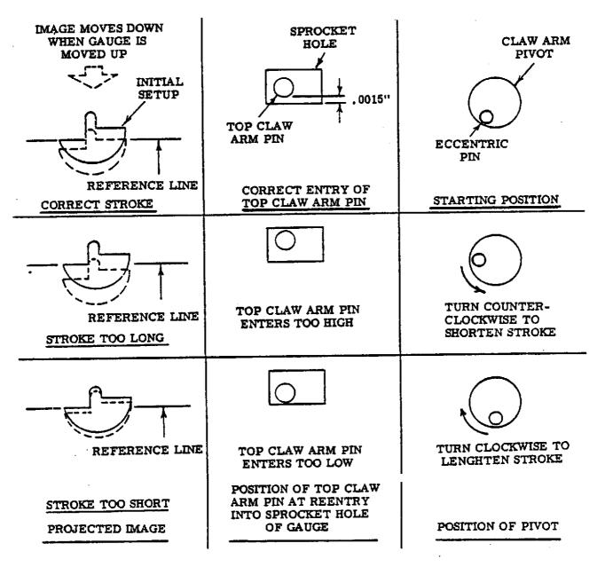
Figure 3-81. CLAW PULL DOWN STROKE ADJUSTMENTS
