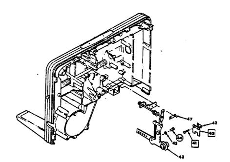
Figure 3-82. FRAMING ADJUSTMENT
