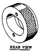
Used to adjust claw arm side clearance and pull-down stroke.
