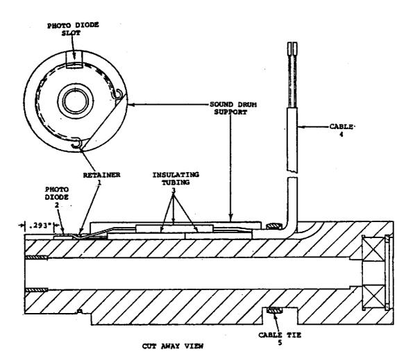
Figure 3-83. REPLACING PHOTO DIODE CHIP IN SOUND DRUM SUPPORT
