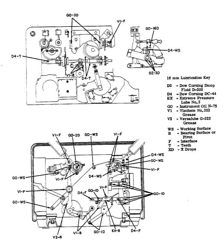
Figure 3-90. PREVENTIVE MAINTENANCE LUBRICATION POINT DIAGRAM
