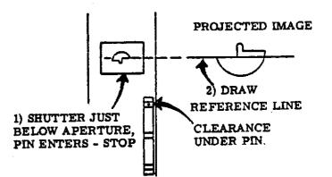
Figure 3-79. CLAW PULL DOWN STROKE SET-UP
