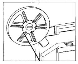
Make sure the film is properly threaded through the channel by turning the take-up reel clockwise with hand.
