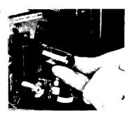
To replace the new exciter lamp, align the three prongs on the socket with the holes on the lamp flange and turn the lamp head clockwise until it locks into place.
