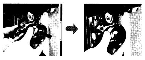
Make sure the lens can move back and forth by turning the focusing knob.
