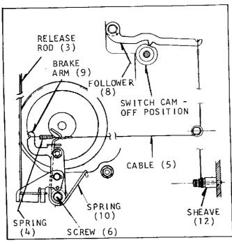
Figure F-1. Brake Component Installation
