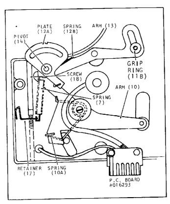
Figure C. Arms and Counterbalance Spring Installed
