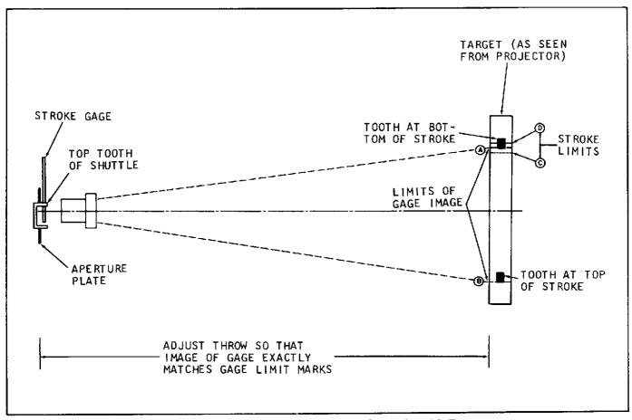
Figure M. Checking and Adjusting Shuttle Stroke with Target
