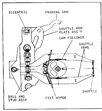
Figure B. Shuttle Arms and Cams Assembled
