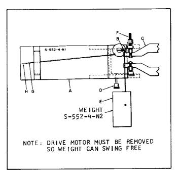
Figure L. Adjusting Fit of Shuttle Arms to Pull-Down Cam
