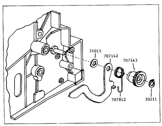
Figure C. Correcting Noisy Reverse Operation
