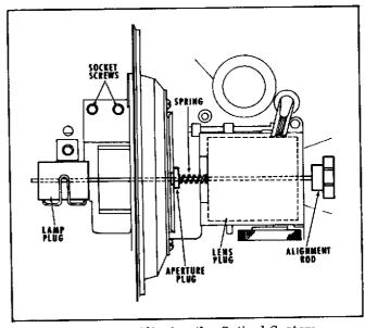
Figure H. Aligning the Optical System
