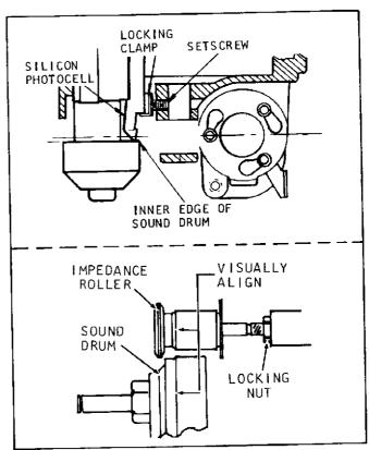
Figure E. Photocell, Sound Drum and Impedance Roller Installation
