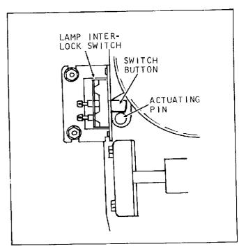
Figure G. Adjusting Lamp Interlock Switch
