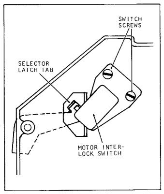
Figure D. Adjusting Motor Interlock Switch
