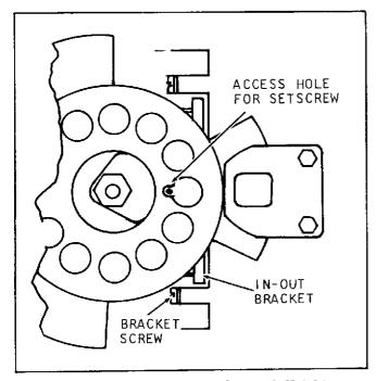
Figure K. Adjusting Shuttle Tooth Height
