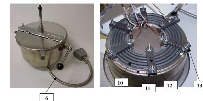
**Important:** Note the position of the thermal couples and the heat element connections. If the kettle is taken apart, these parts must be put back in the same position.
