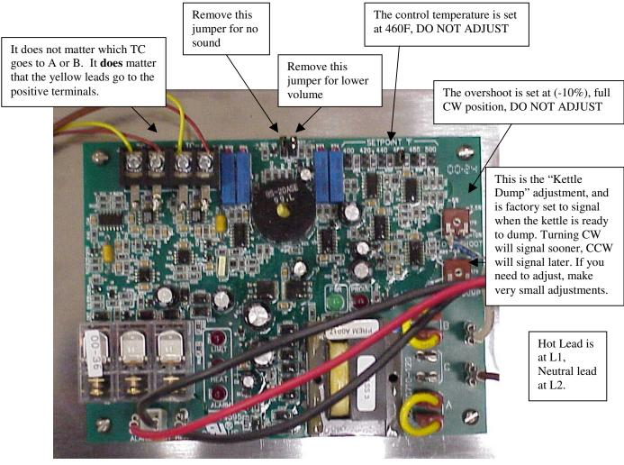
Position for 120v supply (shown) is jumper A and B. For 240v, jumper C only, remove A and B jumpers.
