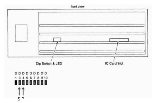
With a good SDDS print played on a fully working SDDS system, these two LED's should be on all the time, apart from through splices. Frequent dark bursts indicate a faulty print or a faulty SDDS system.
