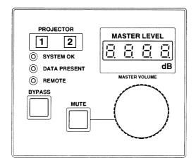
If the Data present indicator is off, the film is not running through the reader at the right speed.
