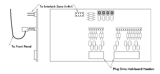
The shield board is now plugged onto the headers on the main circuit board where the connectors used to be. Besides the pins of the header, there is no other mechanical means to mount the Shield, so be careful. Replace the MCU board being sure that there is an insulating layer between the Shield board and the MCU board.
