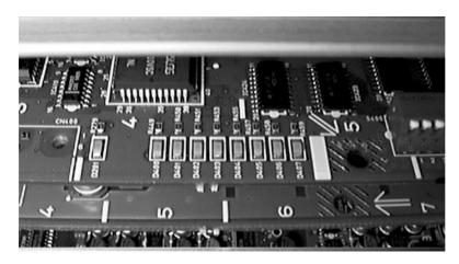
With a good SDDS print played on a fully working SDDS system, these two LEDs should be on all the time, apart from through splices. Frequent dark bursts indicate a faulty print or a faulty SDDS system.
